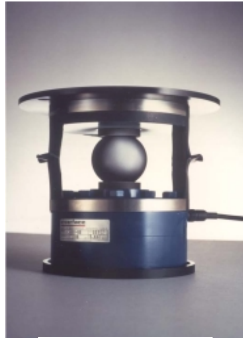
Fig.28 Ball and Socket Method of Isolating Extraneous Loads
