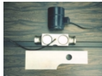
Fig.10 Three Types of 50,000 lb Load Cells
